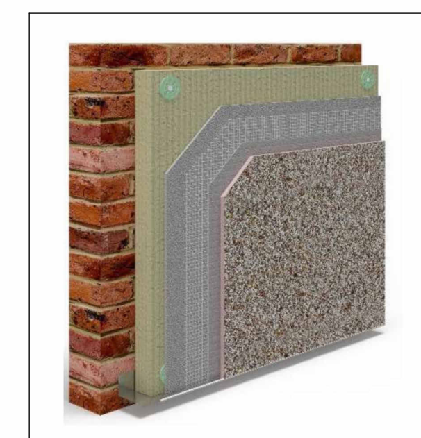
100mm Wetherby Stone Wool insulation with Spar Dash finish (colour to be confirmed by the Client).
