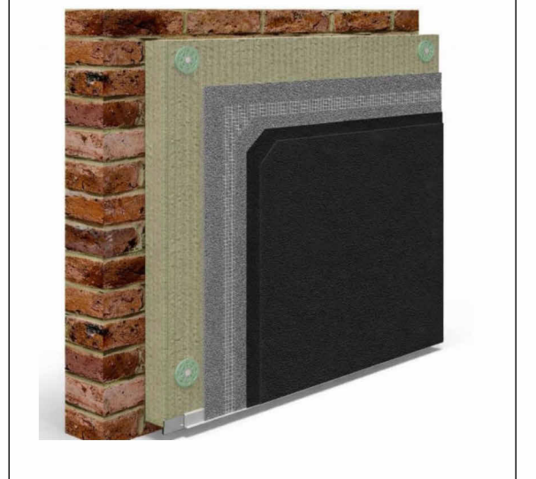
80mm Wetherby HD EPS insulation installed below DPC where required, ensuring \geq 150\text{mm} clearance between finished render and external ground level. Colour to be confirmed by the Client.
